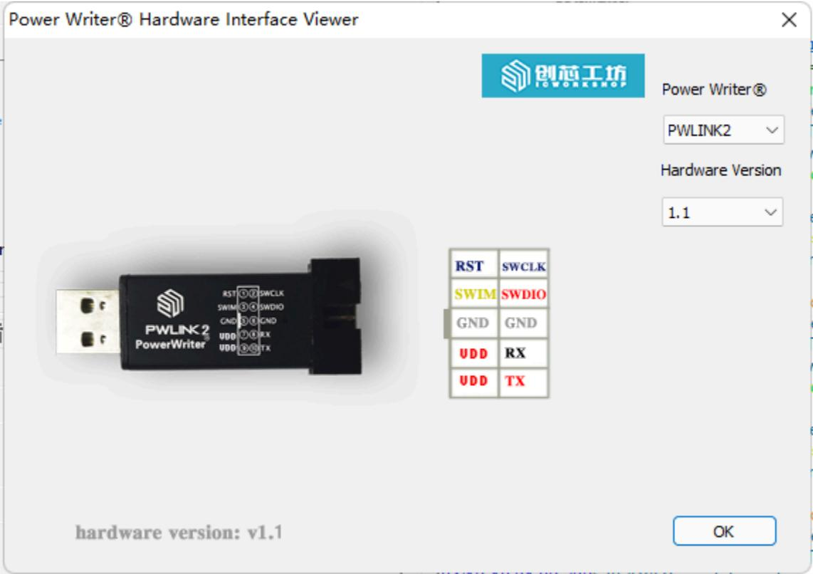
**VREF 5V**: When pins 7 and 9 of PWLINK2 and PWLINK2 Lite are VREF and 5V, the 5V pin only outputs 5V supply voltage, which is not controlled. The operating mode of the Vref pin can be configured by the upper computer, with 3.3V output by default, 5V output mode by the upper computer, or an "input mode" that provides an internal
