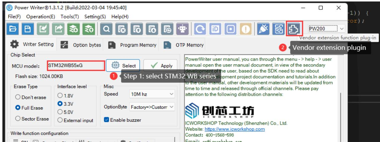
After selecting the STM32WB family of chips, an Extended Functions button appears on the right side of the toolbar, defined as Vendor Specific Plug-In Functions, which can be clicked to enter the STM32WB Protocol Stack programming configuration page, as shown in the figure:
